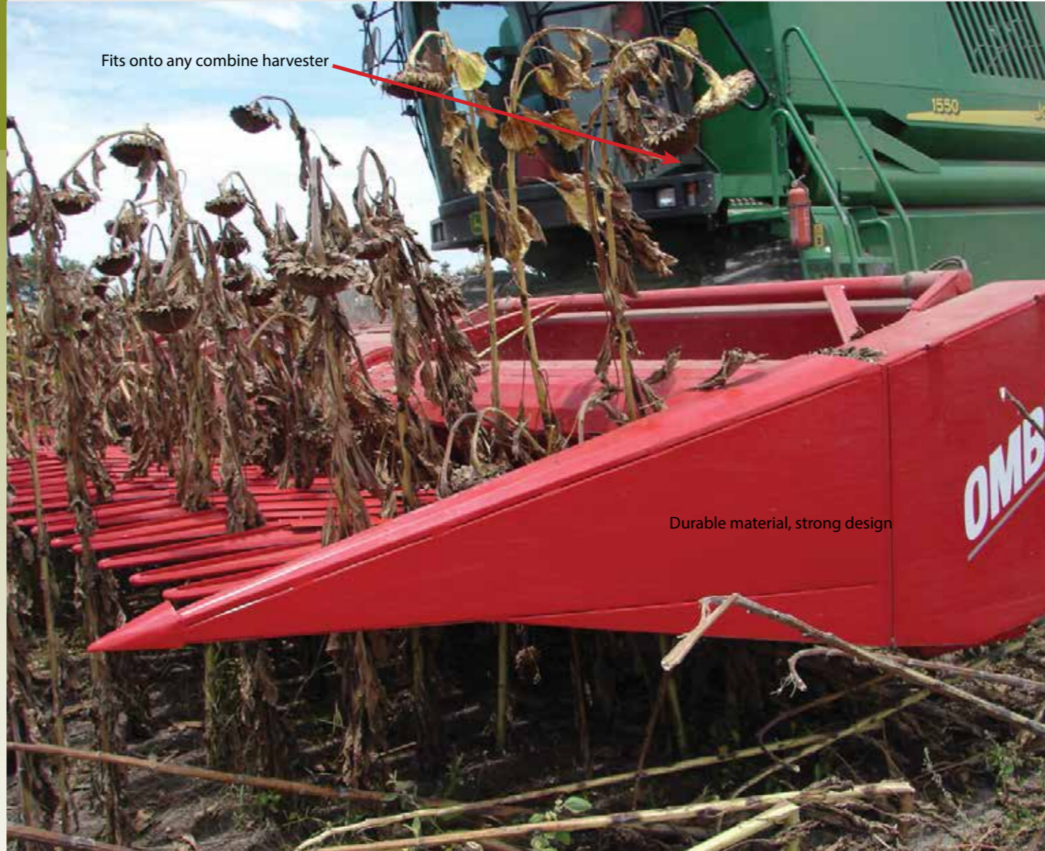
The Ombu sunflower header demands the minimum of combine power and diesel. Its mechanism is easily turned by hand.
