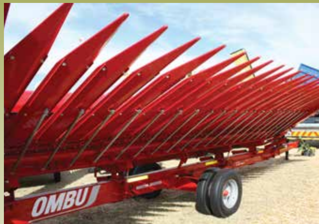
The Ombu sunflower header demands the minimum of combine power and diesel. Its mechanism is easily turned by hand.
