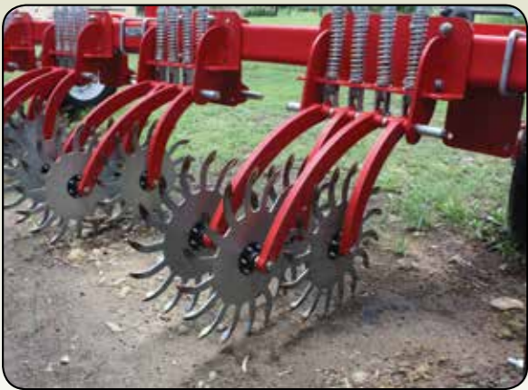
Every roller is mounted on its own spring-loaded arm and 100 mm apart for a working width of 400 mm on the 4 roller or 600 mm on the 6 roller.
