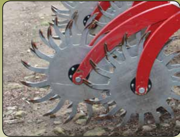
High tensile steel spiked wheels with no joints and rivets.
