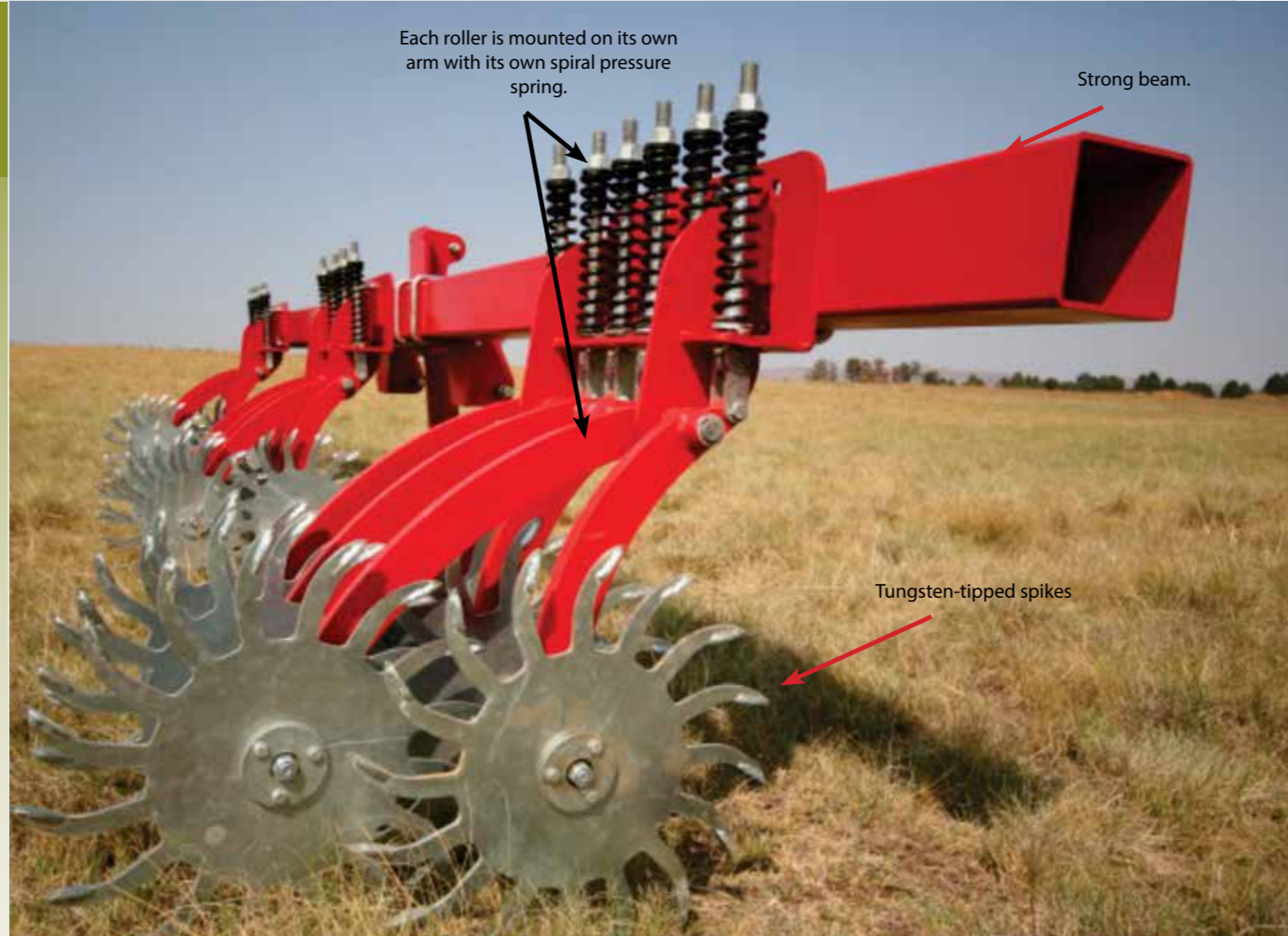
High tensile steel spiked wheels with no joints and rivets.
