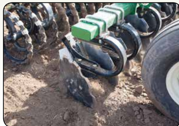
INDIVIDUAL DISC MOUNTS – Offer more space between discs for excellent trash flow and better performance in wet conditions.
