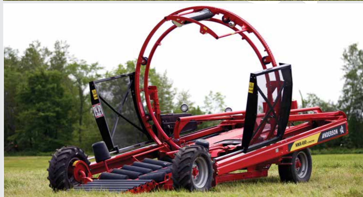
Remote steering starts, stops and steers the bale wrapper without leaving the tractor.
