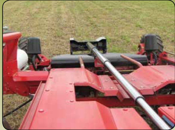
Xtractor push-off system allows for quick and hassle-free push off of the last bale.
