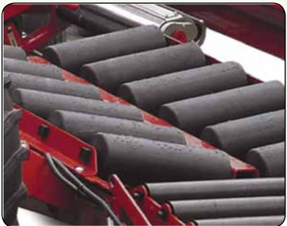
V-shaped floor to accommodate round bales.
