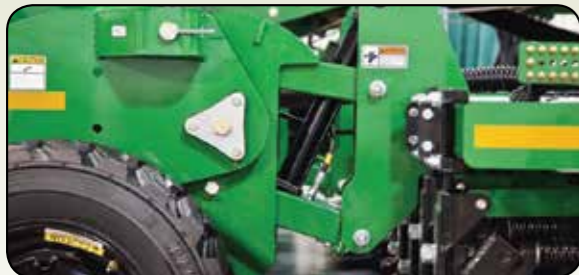
HYDRAULIC DOWN PRESSURE - The NTA-3007 Air Drill features a unique hydraulic down-pressure system which, through parallel linkage, maintains opener-to-ground geometry.
