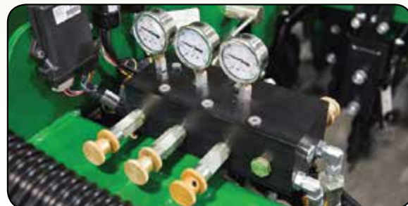
HYDRAULIC WEIGHT TRANSFER - Ensures that all rows have the same amount of weight available for penetration - even when crossing undulations.
