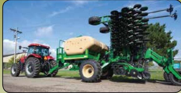
NARROW TRANSPORT - Transport width is just under 3m.
